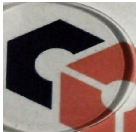
Fig. 5: Photo of a 2.3 \mu m Terefilm film on an optically transparent fused silica disk.
