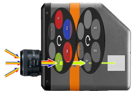
Figure 5 - A CIE-matched tristimulus filter wheel system (shown here inside a ProMetric® I-Series Imaging Colorimeter) enables a measurement device to capture light and color as perceived by the human eye.
