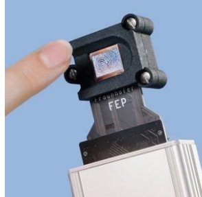
Bidirectional OLED microdisplay as fingerprint sensor © Fraunhofer FEP
