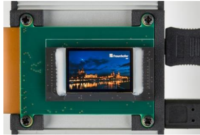
1-inch WUXGA OLED microdisplay © Fraunhofer FEP
