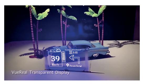
Note that the unique ability of microLEDs to enable tiled displays could prove useful in automotive applications, as companies could produce standard modules and automotive display designers can create custom shaped displays. It remains to be seen whether this is a viable route, though.
